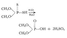
Therefore 1 ml. of 0.1N chloramine-T is equivalent to 2.064 mg. of pure malathion.
